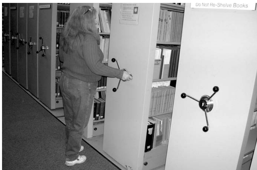
Compact shelving units are compressed together. When the handle is turned they move along tracks, allowing a few wider passages between the tracks.
